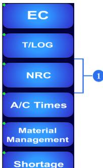
The A/C TIMES application allows users to register aircraft and APU utilization: total and the last flight cycles and hours. To begin to work with this submodule, you need click "A/C Times" button (1) on the right side of the PART M module list. On the left side of window there is A/C - APU Utilization Registration List (2). Here you can see the whole list of aircraft data. On the right side of window there is Editor page (3) for A/C utilization, APU utilization and ETOPS data.
