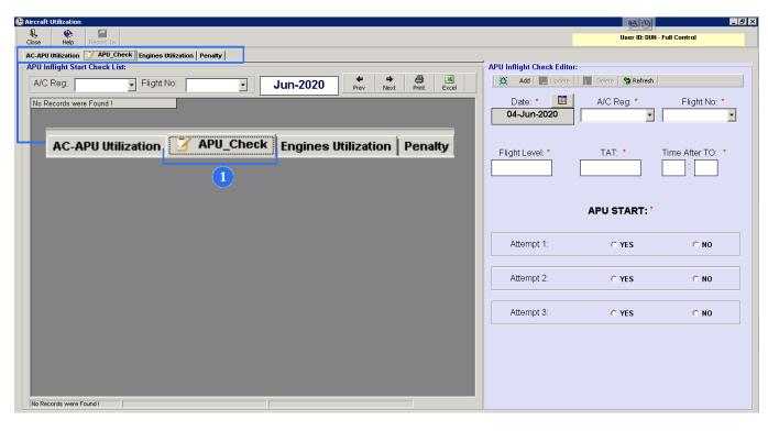
1. APU Check is used to register APU start in flight. To open an APU Inflight Start Check List, click on the APU Check button.
