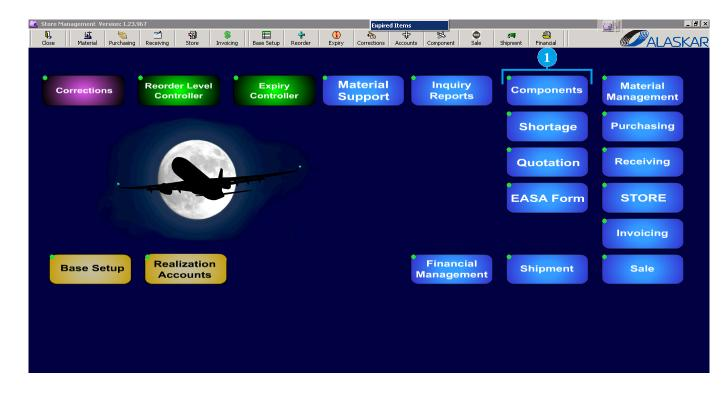
1. A Components Sub-Module maintains all processes connected with components in the company. It allows registering repair and exchange orders, keeping unserviceable items at repair shelf, tracing repair / exchange orders and checking any component's history.
